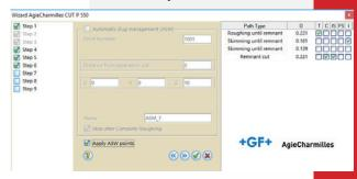
The Die can be fixed anywhere on the geometric path during its Main CUT. To remove the core slug at the end of the main cut a simple knock out will do it. Users can use ASW instead of the typical Remnant cut to achieve better surface quality
